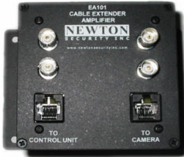
Figure 11 – T-DAR Cable Extender/Amplifier
