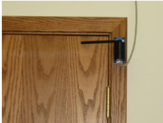
**Figure 39 –Position of Encoder on door**
