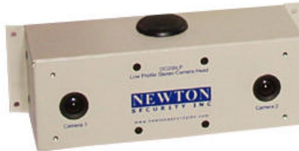
Figure 5 - T-DAR Stereo Tracking Head
